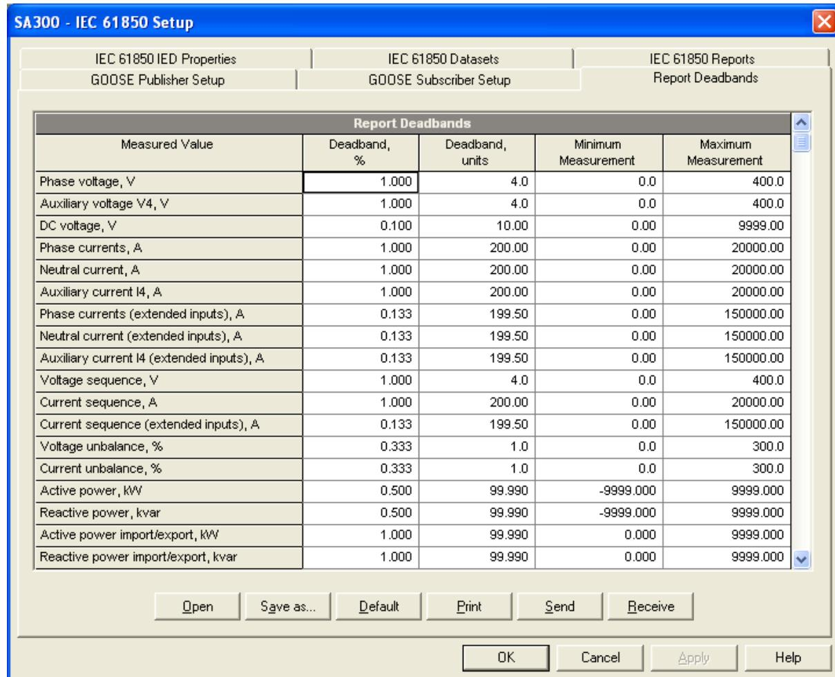
For your convenience, PAS shows the deadbands both in percent and in engineering units, and also indicates the minimum and maximum process measurements from which the percent deadband is taken.
