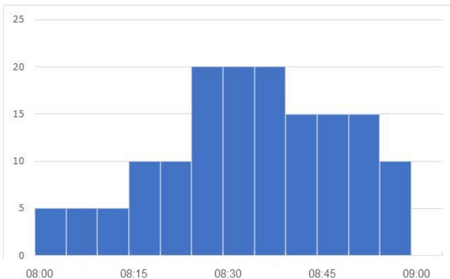
The advantage of this method is its simplicity of calculation and no requirement for external synchronization while the disadvantage is that the results will vary between devices. For example, if another meter will have 5-minute offset in its internal clock the demand in the example above will be 6.6 rather than 5 (from 08:05 to 08:10 and 08:10 to 08:15 the value is 5 and from 08:15 to 08:20 the value is 10, which result  $\frac{5+5+10}{3} = 6.6$ ).
