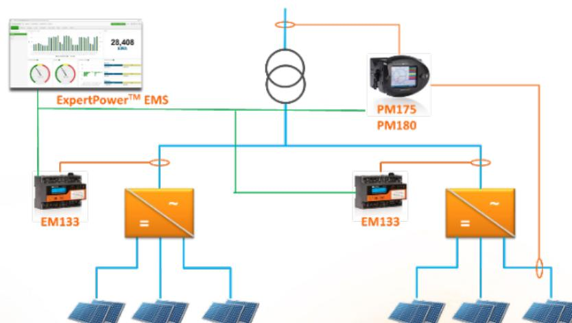
Integrated into an EMS (ExpertPower™, below), the metering points mentioned allow for real-time monitoring of voltage and current measurements and accordingly, real-time monitoring of system capacity.
